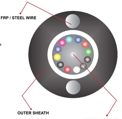
LOOSE TUBE WITH JELLY & FIBRE
